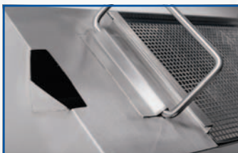
Profiled oil outflow
